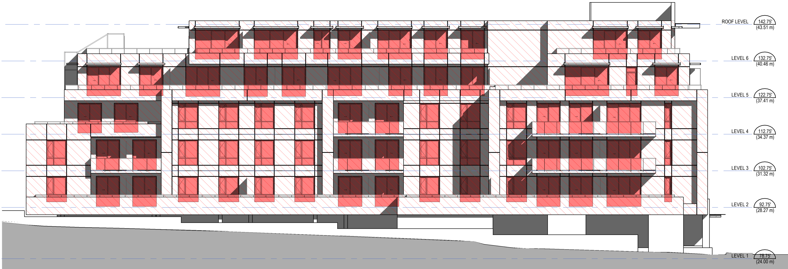
② NORTH ELEVATION - EXPOSING BLDG FACE 1 : 150
